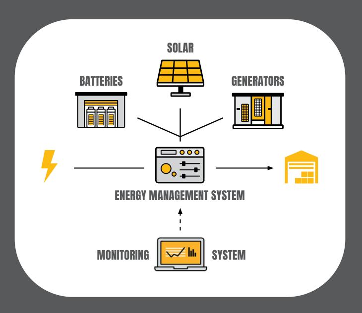
Microgrids are a good and sustainable solution for the current grid congestion, because they are stand-alone power grids into which local, sustainable energy sources are integrated. A microgrid is, as it were, a mini version of the regular electricity grid, but can still be connected to that grid if necessary or desired.
