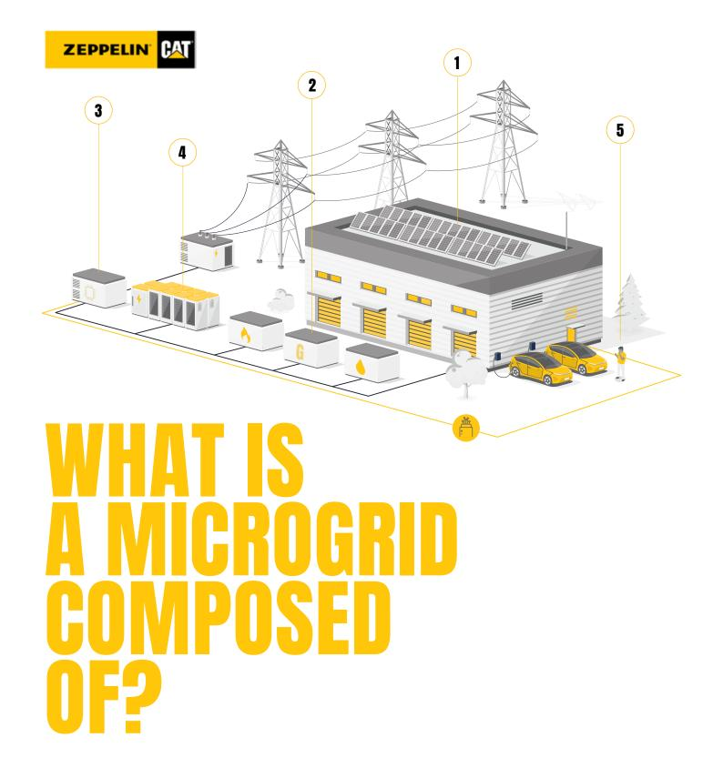
In most cases, a microgrid consists of solar panels, a generator set, Energy Management System for optimal use of grid components, an energy storage system and Cat Connect for remote monitoring. The grid stabilisation module for peak load assistance, the energy timing module for peak load limitation, and the energy capacity expansion module are all part of the energy storage system.
